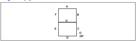
Figure 23. Register Bitmap: 7-Segment Display MSB FE84 0000h (Write Only)
